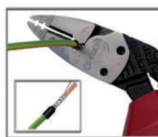
Aderendhülsen crimpen Crimping of ferrules 1,5 - 2,5mm 2
