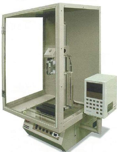
General model for desk testing machine The whole of the moving part is covered. When a window is not closed, there is the safety device which cannot perform movement of the testing machine.
