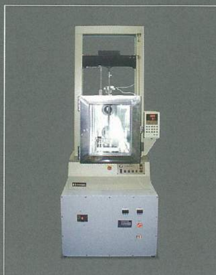
Constant Temperature Chamber finished
